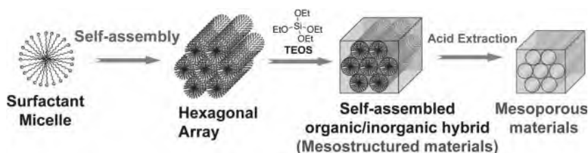
Figure 12.1 Formation mechanism of mesoporous silica materials.
