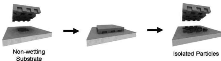
Figure 10.6 Schematic drawing of the PRINT process. A solvated precursor is compressed between a nonwetting substrate and a PFPE mold. The procedure produces isolated
